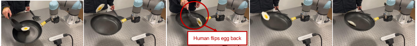
Fig. 9: Human Perturbation Robustness. This figure showcases the robot’s ability to handle human-induced perturbations across three tasks: (1) In nail hammering, the robot successfully followed a manually moved nail; (2) In meatball scooping, it located and scooped meatballs even when additional ones were thrown into the pan mid-task; and (3) In egg flipping, the robot consistently flipped the egg back after human intervention repositioned it. These results highlight the policy’s robustness to unpredictable human perturbations.
