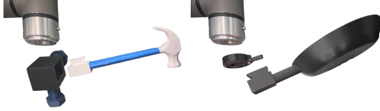
Fig. 11: Fast Tool Changer . Two designs are shown: the left accommodates general tools with a screw mechanism, and the right clips onto tools with specific mounting shapes.
